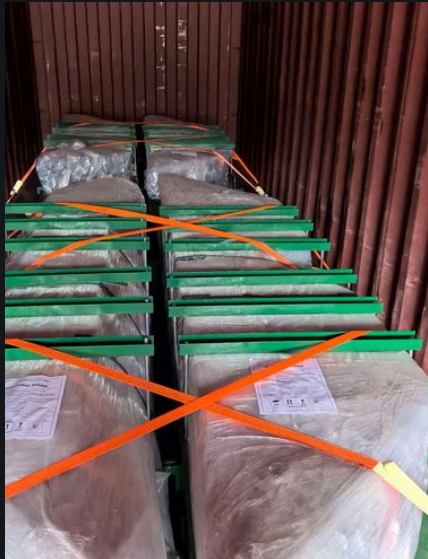
02 Restraint Frames, cases and lashing sized to hold core geometry under load.
