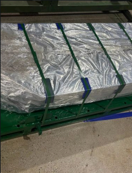
01 Protection Moisture barrier, desiccant and edge protection for the product, season and sea route.
