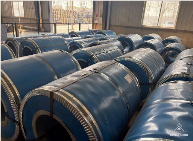
FIG 13 CRGO COILS — PROTECTED IN THE MATERIAL STORE
