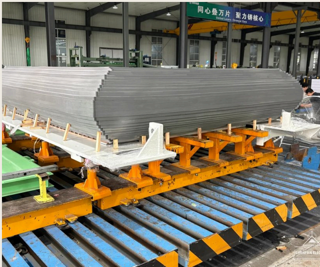
FIG 04 STAGE 04-05 — STACKED LIMB ON THE ASSEMBLY CRADLE
