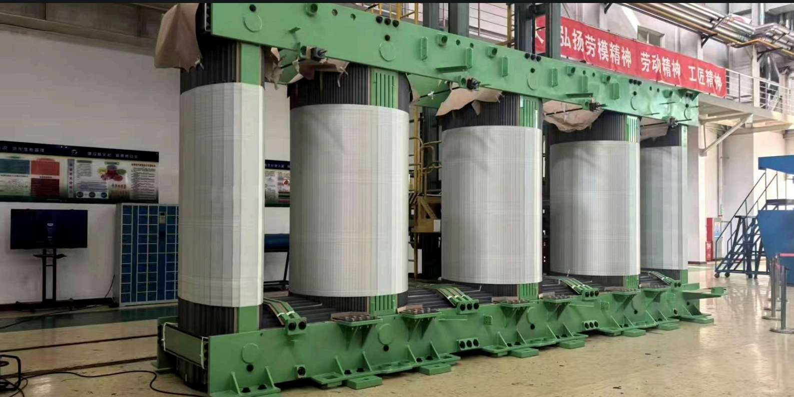
FIG 12 LARGE FIVE-LIMB TRANSFORMER CORE WITH CLAMPING FRAMES — ASSEMBLED IN THE WORKSHOP
