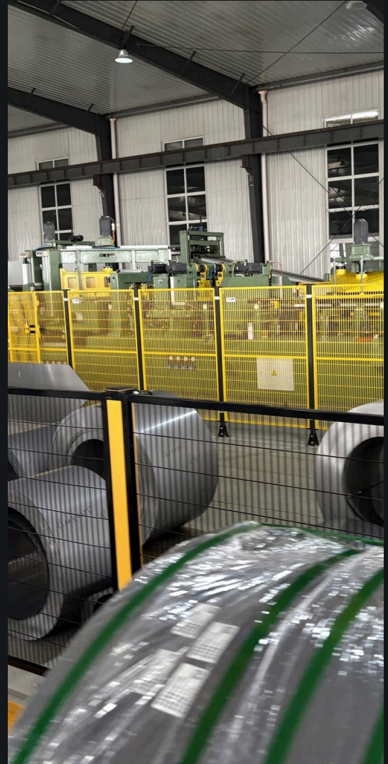
FIG 07 SLITTING LINE — STRIP COILS IN PRODUCTION
